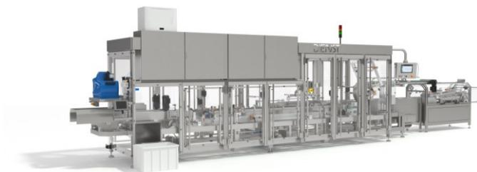
It includes full-length doors so that everything is easily visible and malfunctions can be rectified quickly and effectively. Less time is also required for maintenance work. We have installed a new infeed version with pneumatic overload function and automatic return of the pushers. This is also integrated in the standard version.
